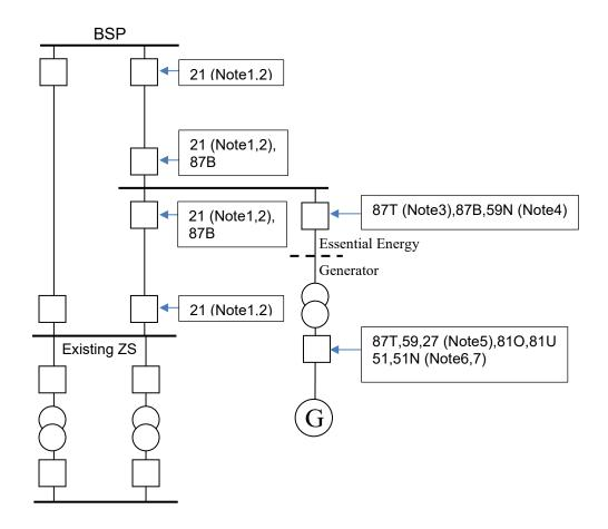
Note1: Where the subtransmission feeder is >100kV then duplicated communicated assisted distance or line differential will be required instead of distance. If single communications are used protection will need to meet NER clearing times for loss of communications.
