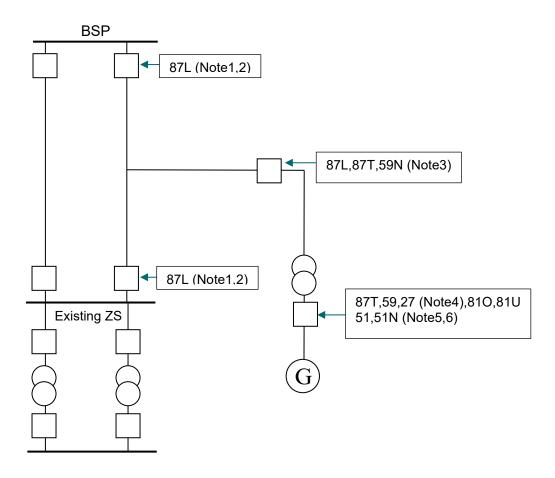
Note1: Where the subtransmission feeder is >100kV then duplicated line differential with duplicated communications are required.
