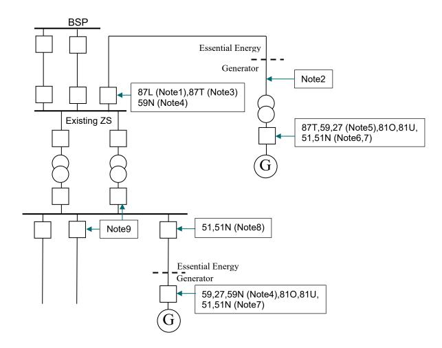
Note1: Where the feeder is >100kV then duplicated line differential with duplicated communications is required. If <100kV then duplicated communications advised.
