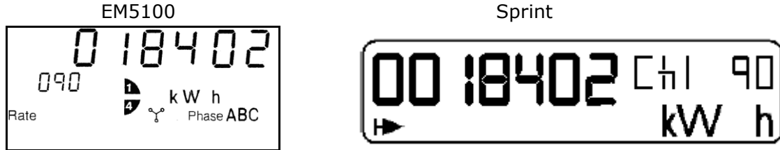
eg The display indicating 18402 kWh – controlled load
