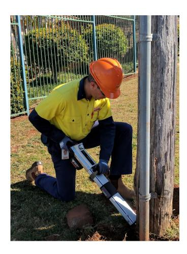
**Suggested caption:** The hand-held wood inspection drill is easier to handle for Essential Energy asset inspectors and will deliver productivity and efficiency gains.
