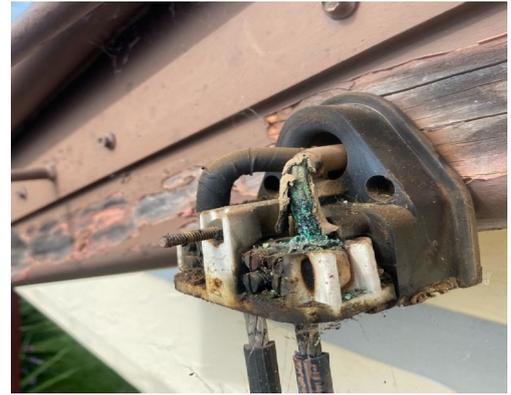
Figure 12 High impedance neutral identified through the trial
