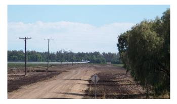
Buildings such as houses and sheds are likely to have power connected through overhead structures. Roads may provide a convenient corridor for powerlines and by identifying at least two poles, pilots can gauge the path of the wire.
