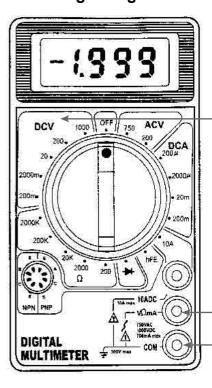
Turn the meter to the DCV quadrant depending on your voltage supply. Start at 20V then work down through the dial until you get a reading that makes sense on the display. Remember 2000 m is representing 2000 millivolts or 2V while 200 m is measuring 0.2V. Most batteries are 1.5V.
