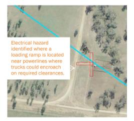
Above: This example shows a loading ramp that is located near overhead powerlines, potentially exposing vehicle operators to electrical hazards\*
